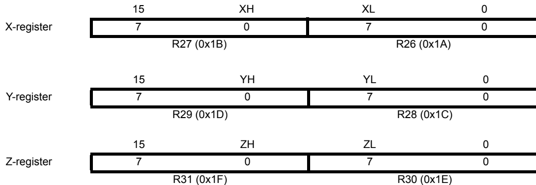
Figure 6-3. The X-, Y-, and Z-registers
